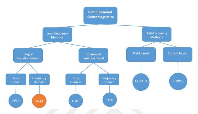
Figure 2.1: A flow chart showing different computational electromagnetic techniques.
