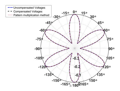
Figure 3.36: Radiation pattern of three element triangular array in xy-plane at 300 MHz with uniform excitation.
