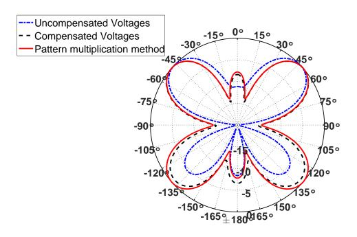
Figure 3.39: Radiation pattern in xy-plane for a 3-Dimensional dipole array at 300 MHz.
