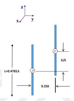
Figure 3.4: Two identical parallel dipole antennas in staggered arrangement with length  $L = 0.4781\lambda$ , radius  $a = 0.001\lambda$ , fixed horizontal separation of  $0.25\lambda$ , and staggered by  $h/\lambda$ .
