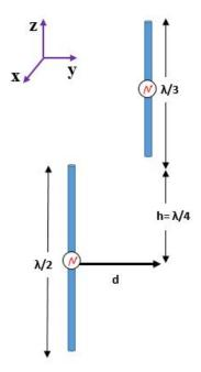
Figure 3.17: Two parallel dipole antennas of lengths  $\lambda/2$  and  $\lambda/3$  in staggered arrangement as a function of spacing relative to wavelength with  $a = 0.001\lambda$ , horizontal separation d and staggered by  $h = \lambda/4$ .
