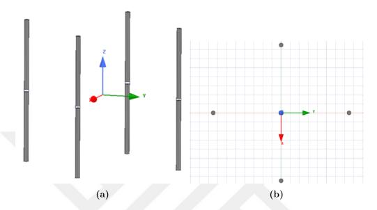
Figure 1.1: Circular array of four half-wave dipoles with radius of circle  $\lambda/4$ . a) Side View. b) Top View.
