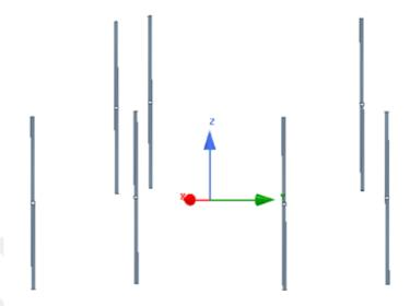
Figure 3.38: Three-dimensional dipole array with seven elements. Four dipoles are placed along a circle of radius  $0.5\lambda$  and three dipoles along a radius of  $0.4\lambda$  which are displaced in the z-axis by  $h = \lambda/4$ .
