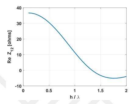
Figure 3.5: Real part of mutual impedance between two identical but staggered dipole antennas of length  $L = 0.4781\lambda$ , radius  $a = 0.001\lambda$ , fixed horizontal separation of  $0.25\lambda$ , and staggered by  $h/\lambda$ .
