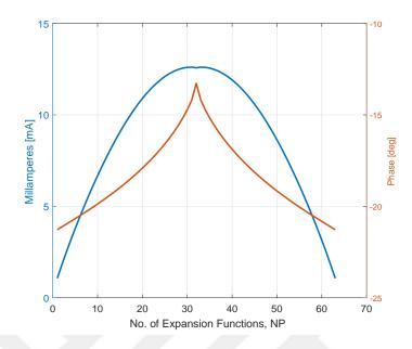
Figure 2.4: Magnitude and phase of the current distribution for a center-fed dipole in free space with length  $L = 0.4781\lambda$ , radius  $a = \lambda/1000$  and number of expansion functions NP = 63.
