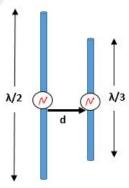
Figure 3.15: Two parallel dipole antennas in non-staggered arrangement of lengths  $\lambda/2$  and  $\lambda/3$  as a function of spacing relative to wavelength with radius  $a = 0.001\lambda$ .
