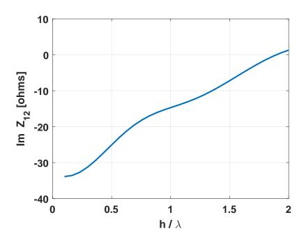
Figure 3.6: Imaginary part of mutual impedance between two identical but staggered dipole antennas of length  $L=0.4781\lambda$ , radius  $a=0.001\lambda$ , fixed horizontal separation of  $0.25\lambda$ , and staggered by  $h/\lambda$ .
