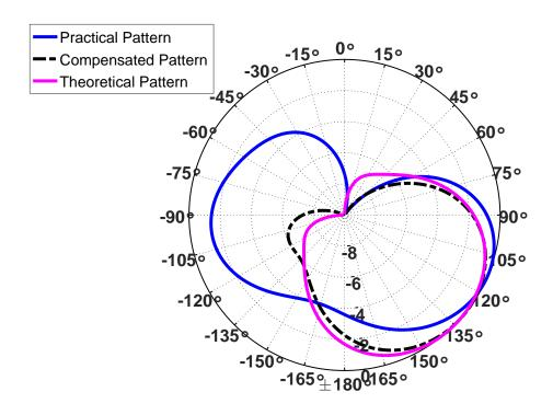
Figure 1.5: Radiation pattern of a circular array of four dipoles.
