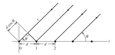
Figure 2.5: Equally spaced linear array of isotropic point sources [1].
