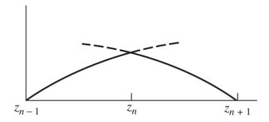
Figure A.5: Piecewise sinusoidal expansion function [1].
