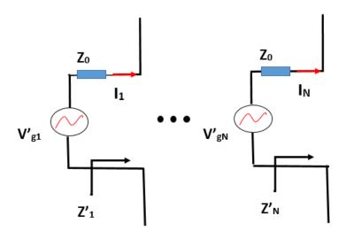
Figure 2.7: Equivalent circuit of N antennas with mutual coupling
