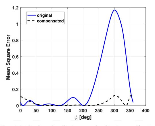
Figure 3.48: Mean Square Error for the compensation of circular array of four dipoles.
