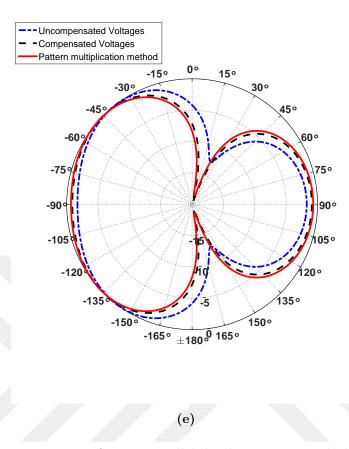
Figure 3.11: Radiation patterns for two parallel dipole antennas with different element separations. (a)  $d = 0.1\lambda$  (b)  $d = 0.2\lambda$  (c)  $d = 0.3\lambda$  (d)  $d = 0.4\lambda$  (e)  $d = 0.5\lambda$ .
