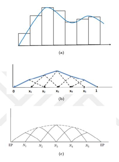
**Figure A.4:** Expansion functions. a) "Staircase" approximation to an actual current distribution. b) Set of overlapping triangular functions. c) Set of overlapping piecewise sinusoidal functions [1].
