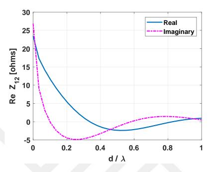
Figure 3.20: Mutual impedance curves for two dipole antennas of lengths  $\lambda/2$  and  $\lambda/3$  in a collinear arrangement with radius  $a = 0.001\lambda$ .
