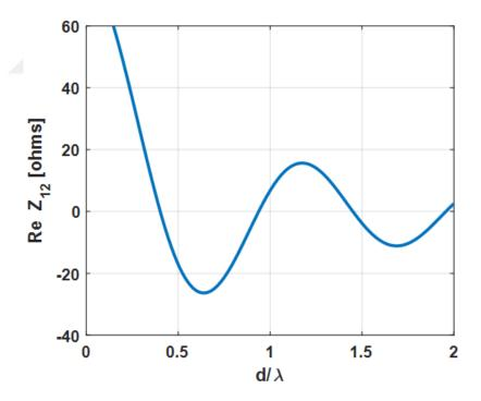
Figure 3.2: Real part of mutual impedance between two parallel dipole antennas as a function of spacing relative to wavelength with  $L = 0.4781\lambda$  and  $a = 0.001\lambda$ . Geometry shown in Fig. 3.1
