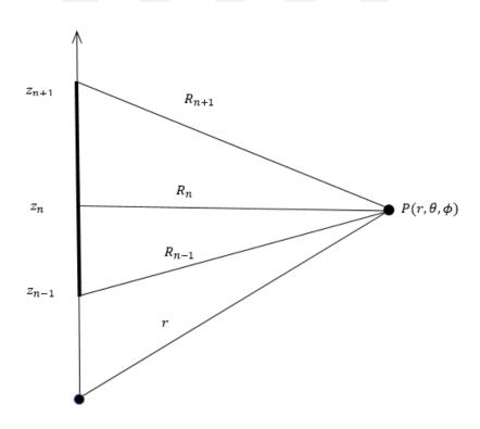
Figure B.1: Wire segment along z-axis [2].
