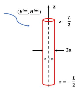
**Figure A.1:** A wire scatterer of length L and radius a illuminated by an incident plane wave.
