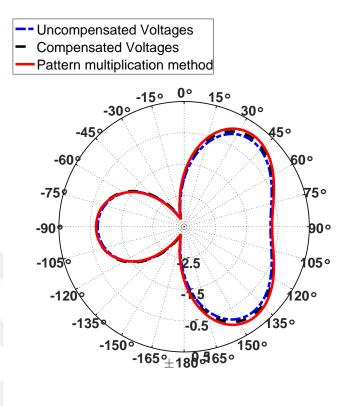
Figure 3.24: Radiation pattern of two-element non-identical staggered dipoles with different element separations. (a)  $d = 0.1\lambda$  (b)  $d = 0.2\lambda$  (c)  $d = 0.3\lambda$  (d)  $d = 0.4\lambda$  (e)  $d = 0.5\lambda$ .
