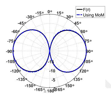
Figure 2.2: Normalized E-plane pattern of a half-wave dipole.
