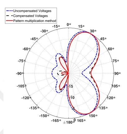
Figure 3.14: Radiation pattern for five-element dipole array with separation  $d = 0.3\lambda$  and mainbeam direction  $\varphi = 60^{\circ}$ .
