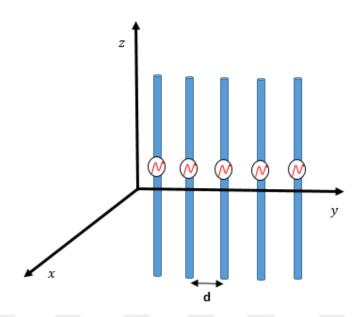
**Figure 3.12:** Five dipole antennas of length  $\lambda/2$ ,  $a = \lambda/200$  and spacing d.
