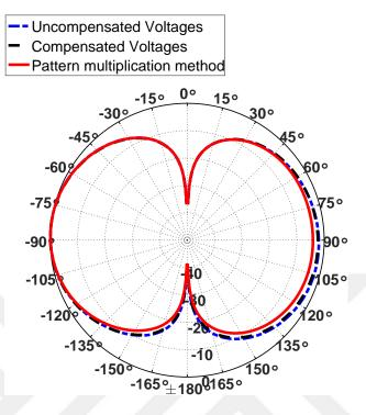
Figure 3.28: Radiation pattern of three element staggered array in yz-plane at 300 MHz.
