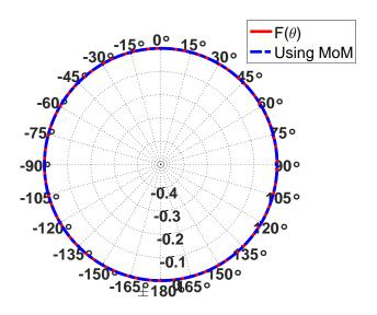
Figure 2.3: Normalized H-plane pattern of a half-wave dipole.
