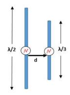
Figure 3.21: Two parallel antennas in non-staggered arrangement of lengths  $\lambda/2$  and  $\lambda/3$  as a function of spacing relative to wavelength with radius  $a = 0.001\lambda$ , and separation d.
