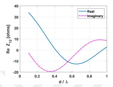
Figure 3.16: Mutual impedance curves between two parallel antennas in non-staggered arrangement of lengths  $\lambda/2$  and  $\lambda/3$  as a function of spacing relative to wavelength with  $a = 0.001\lambda$ .
