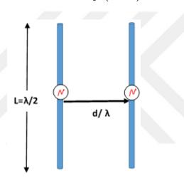
**Figure 3.10:** Two parallel antennas of length  $\lambda/2$  with  $a = \lambda/200$ .
