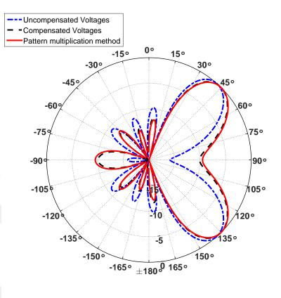
Figure 3.13: Radiation pattern for five-element dipole array with separation  $d=0.5\lambda$  and main-beam direction  $\varphi=45^{\circ}$ .
