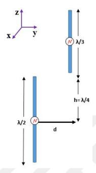
Figure 3.23: Two parallel dipole antennas of lengths  $\lambda/2$  and  $\lambda/3$  in staggered arrangement as a function of spacing relative to wavelength with radius  $a = 0.001\lambda$ , and staggered by  $h = \lambda/4$ .
