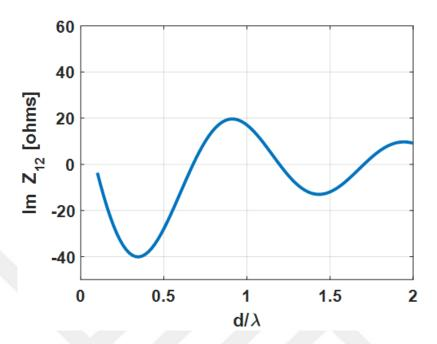
Figure 3.3: Imaginary part of mutual impedance between two parallel dipole antennas as a function of spacing relative to wavelength with  $L = 0.4781\lambda$  and  $a = 0.001\lambda$ . Geometry shown in Fig. 3.1.
