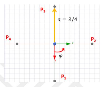
Figure 1.2: Four isotropic sources arranged in a circular array.
