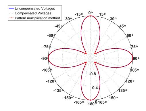
**Figure 3.31:** Radiation pattern of four element circular array in XY plane at 300 MHz with uniform excitation.
