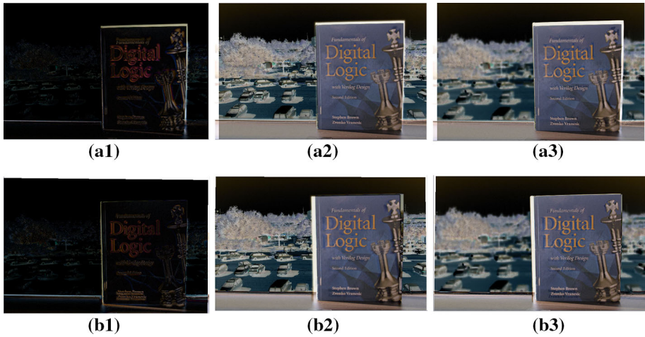
Fig. 7 Absolute difference values between the reference image and the target images after spatial registration with alternative registration methods. a1–a3 MTB alignment. b1–b3 Hugin alignment. These alignment methods are included in the Luminance HDR software [ http://qtpfsgui.sourceforge.net ], and the results are obtained directly using this software
