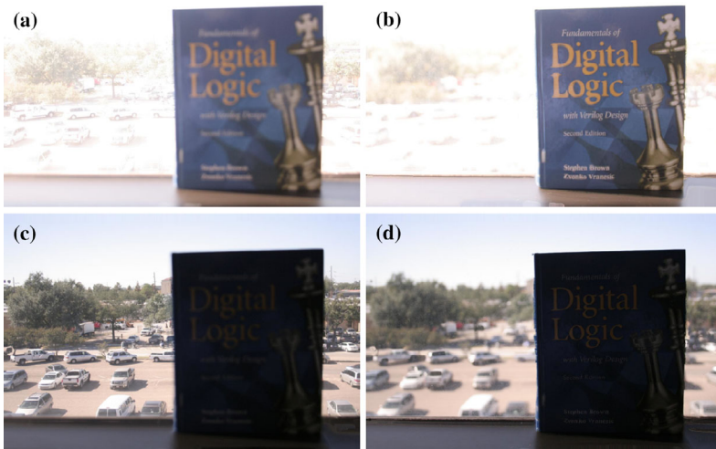
Fig. 5 Spatially registered images. a Original reference image from Fig. 3a; b–d Spatially registered target images from using the estimated motion vectors given in Fig. 4
