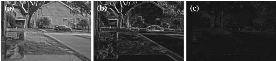
Fig. 15 Absolute difference between the reference and target image before/after registration. a Difference before registration. b Difference after photometric registration. c Difference after photometric and spatial registration
