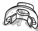
FIGURE 2. Regulator mouthpiece. Mouthpiece of the second stage is a factor in TMJ disorders (A, vestibular shield; B, interdental bite platform; C, palatal flange; D, connector tube to the demand valve of the second stage; arrows, air passing from the demand valve of the second stage to the respiratory tract of the diver through the airway of the connector tube).
