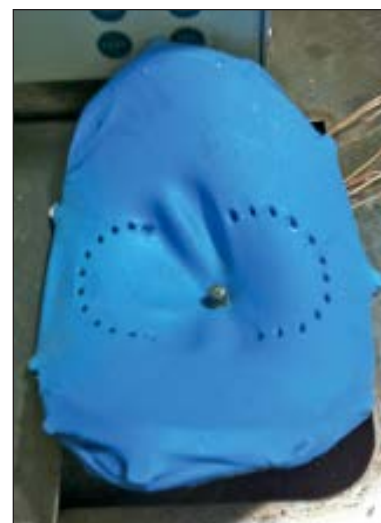
Fig 3 Experimental setup with a rubber dam at the cervix of the abutment and immersed in the thermostatically controlled water bath at 38°C.
