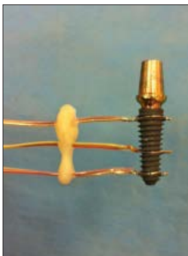
Fig 1 Type K thermocouples twisted around the cervical, middle, and apical parts of a titanium implant with a diameter of 4 mm and a length of 11.5 mm.
