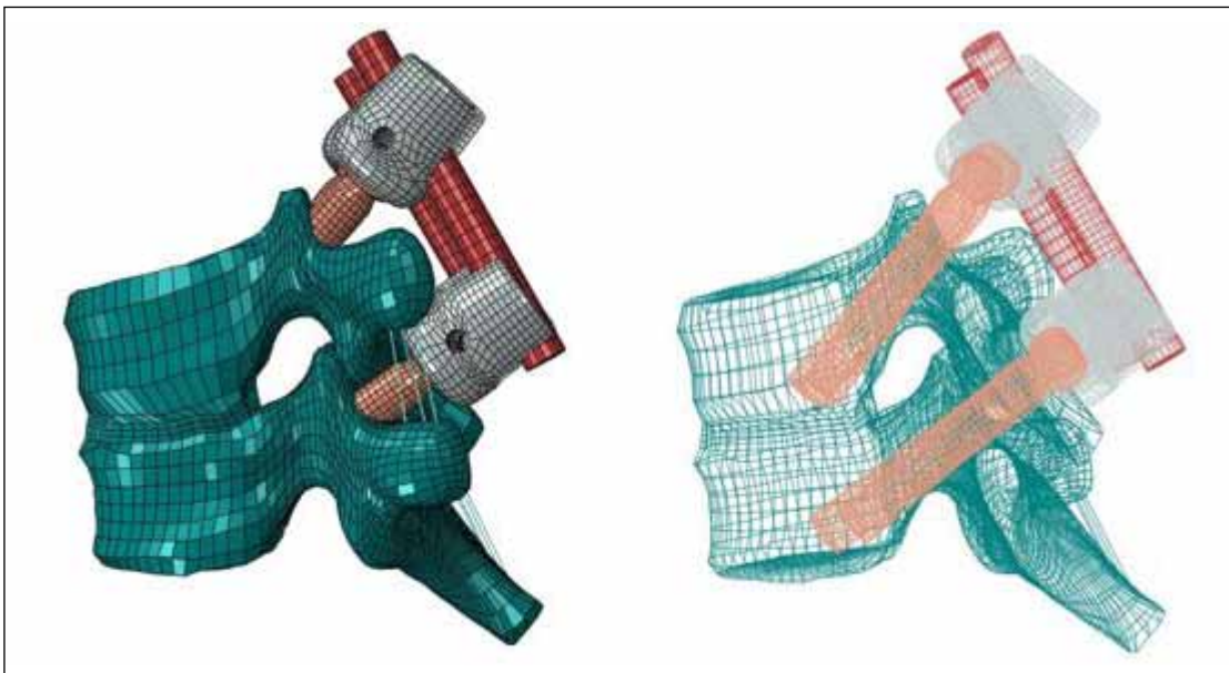
Figure 2: Anatomic Trajectory: FEA model of the T8-9 thoracic spine with pedicle based posterior stabilization system; pedicle screw trajectory parallel to pedicle.
