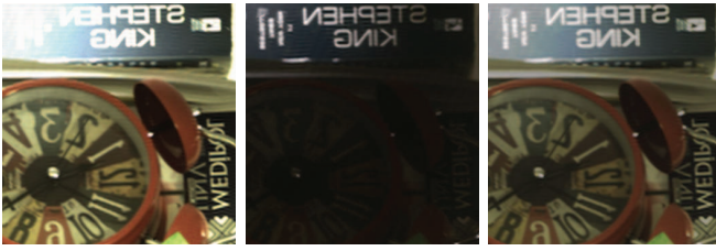
Figure 3: (Left) High exposure image. (Middle) Low exposure image. (Right) HDR image.
