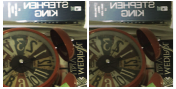
Figure 4: (Left) HDR image without optical mask. (Right) HDR image with optical mask.
