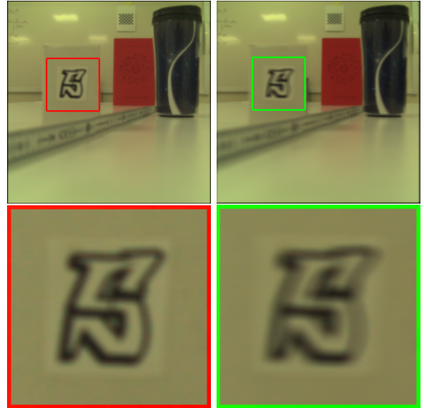
(c) Single light field. Focus is on the back object, the front object is zoomed-in. (d) Four light fields. Focus is on the back object, the front object is zoomed-in.
