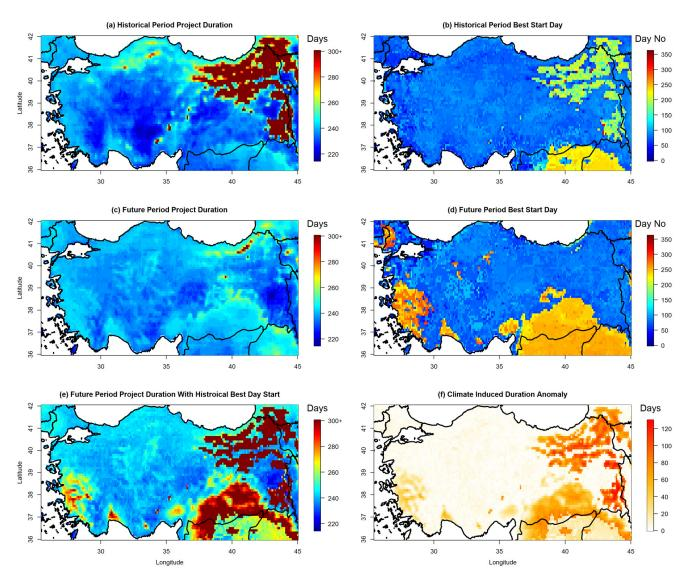
**Figure 8.** Historical (1961–2014) and future period (SSP5-8.5 2071–2100) shortest project duration (**a**,**c**), optimal project start date (date of the year to achieve the shortest duration—**b**,**d**) and future project duration if climate change effects are not considered (**e**,**f**).
