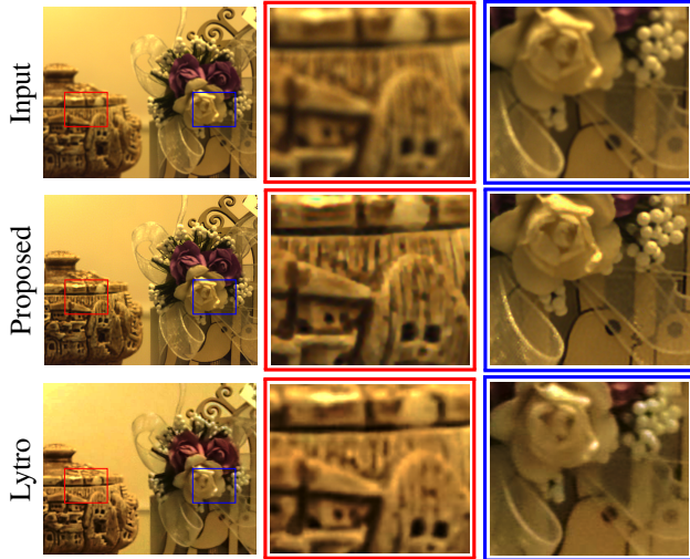
Fig. 6: Comparison of light field perspective image recovered by the proposed method and captured by a Lytro camera. Input image is the wide aperture image used by the proposed method.
