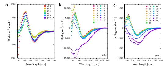
**Figure 2.** (**a**) MRE values for trastuzumab within different pH at 20 °C. (**b**) Temperature-ramped CD spectrum of trastuzumab at pH 4 and (**c**) pH 9.
