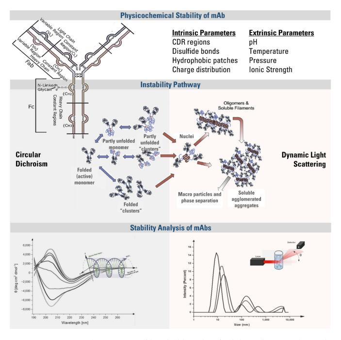
**Scheme 1.** Overview of thermal stability analysis of mAbs by complementary tools: CD and DLS (instability pathway image was adapted from Ref. [3], and IgG1 structure was adapted from Ref. [9]).
