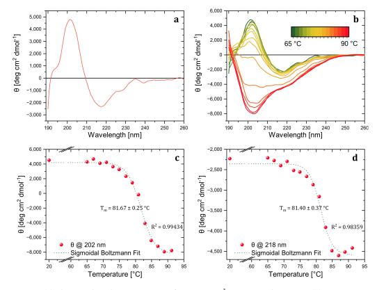
**Figure 1.** (a) The wavelength CD spectrum of 0.2 mg·mL<sup>-1</sup> trastuzumab at 20 °C. (b) Temperaturewavelength CD spectrum of 0.2 mg·mL<sup>-1</sup> trastuzumab between 65–90 °C by 2 °C intervals at 218 nm (c) Denaturation curve of trastuzumab at 202 nm. (d) Denaturation curve of trastuzumab at 218 nm.
