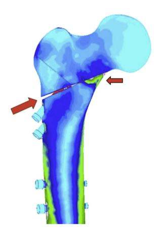
Fig. 4. Single leg standing position caused displacement at the fracture site.
