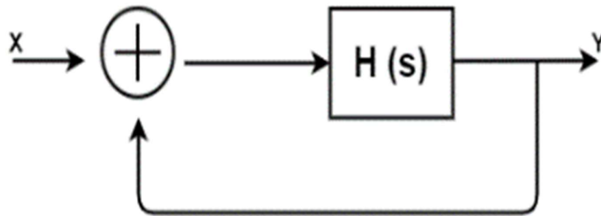
Figure 2.3: A simple feedback system.
