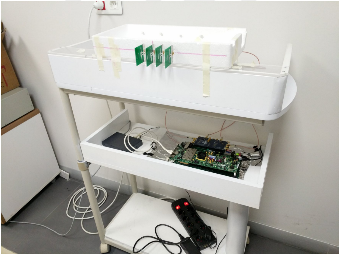
Figure 4.19: A commercial quasi yagi array for estimating DoA for different spacings.
