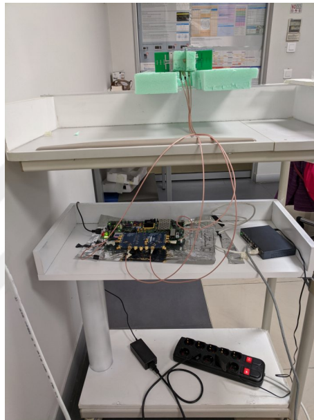
Figure 4.39: UCA of quasi yagi antennas arranged at radius \lambda/4 a) top view, b) bottom view, c) complete setup.
