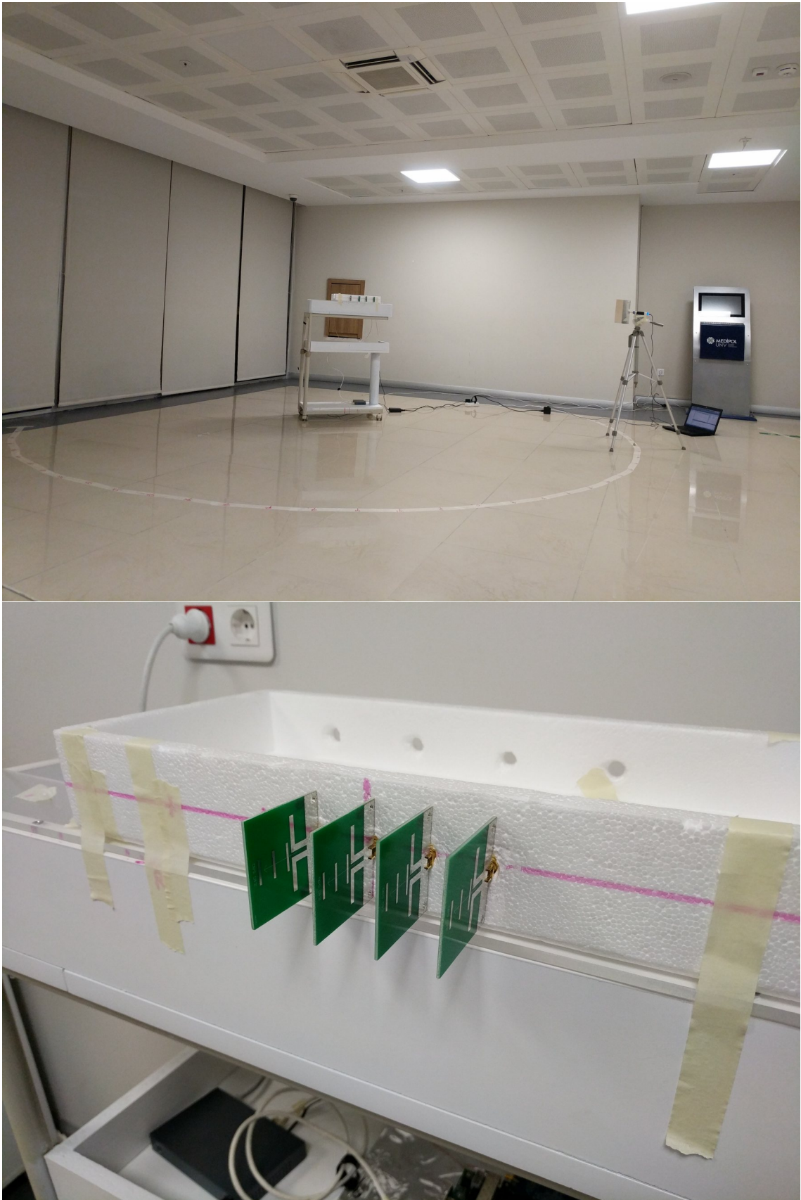
Figure 4.18: A commercial quasi yagi ULA of four-elements with different spacing.
