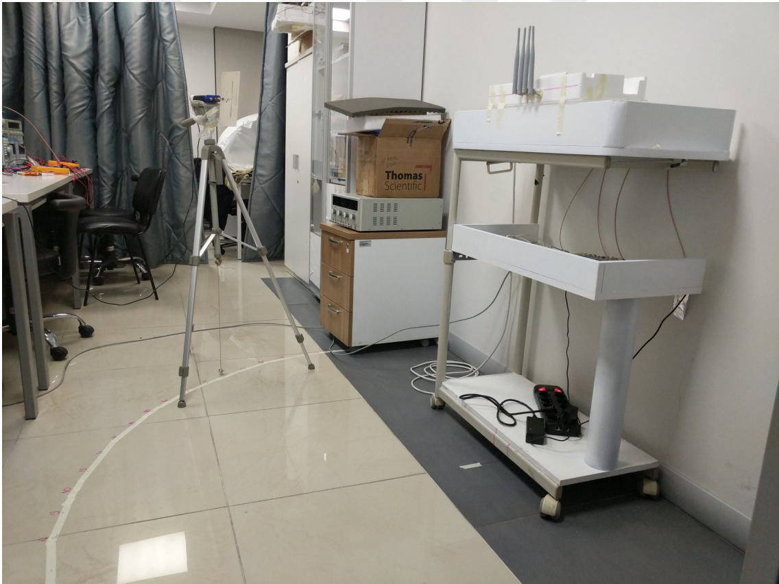
Figure 4.7: Omni-directional four element ULA using TPLink WiFi antennas with spacing 0.24\lambda with a directional antenna as transmitter.
