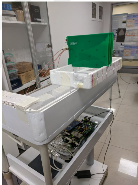
Figure 4.37: Different antenna arrays used for this experiment a) fractal antennas at f=1 GHz and d = 0.33\lambda , b) vivaldi antennas at f=3.7 GHz and d = 0.28\lambda , c) circular patch antennas at f=4.55 GHz and d = 0.37\lambda , d) wideband vivaldi antenna at f=5.95 GHz and d = 0.4\lambda ULA.
