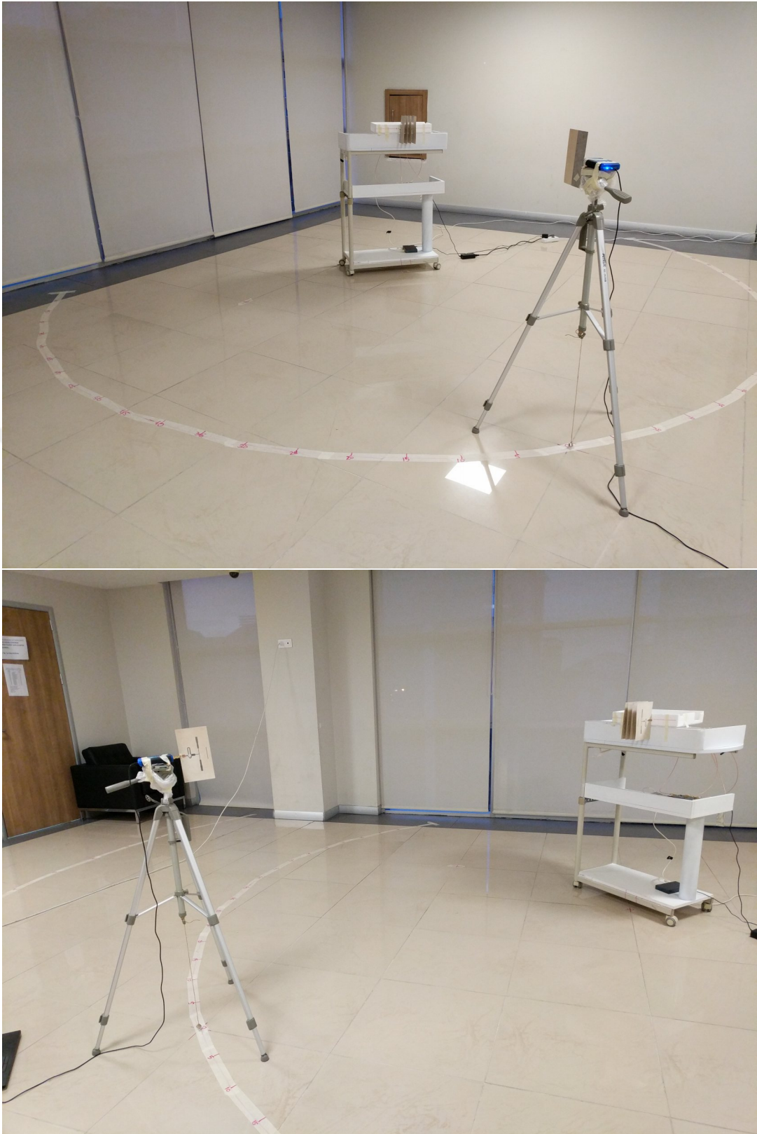
Figure 3.18: DoA testing setup consisting of the transmitter placed on a semi-circle with angles from -90^\circ to +90^\circ with 5^\circ spacing and origin defined at 0^\circ .
