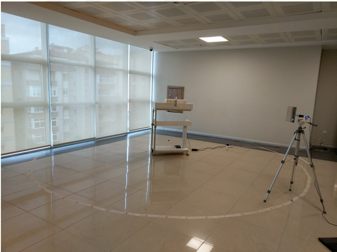
Figure 3.25: Setup for measuring the isolated voltages for the quasi yagi antenna array.
