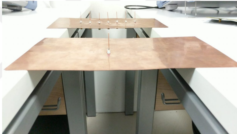
Figure 3.1: A seven-element monopole ULA a) designed and simulated in CST, b) fabricated isolated monopole and monopole array.
