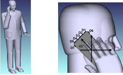
Fig. 2: (left) Human model and (right) location and rotation of PDs on the cell phone
