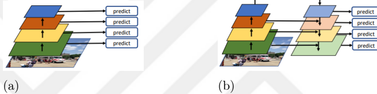
Figure 4.2.2. The types of feature pyramid: (a) Prediction pyramid, (b) Integrated prediction pyramid [9].
