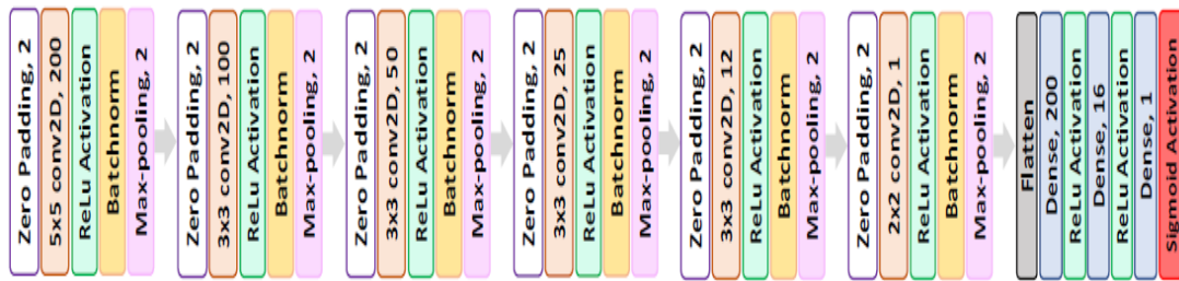
Figure 3.3.2. Low-complexity architecture adopted from [5].
