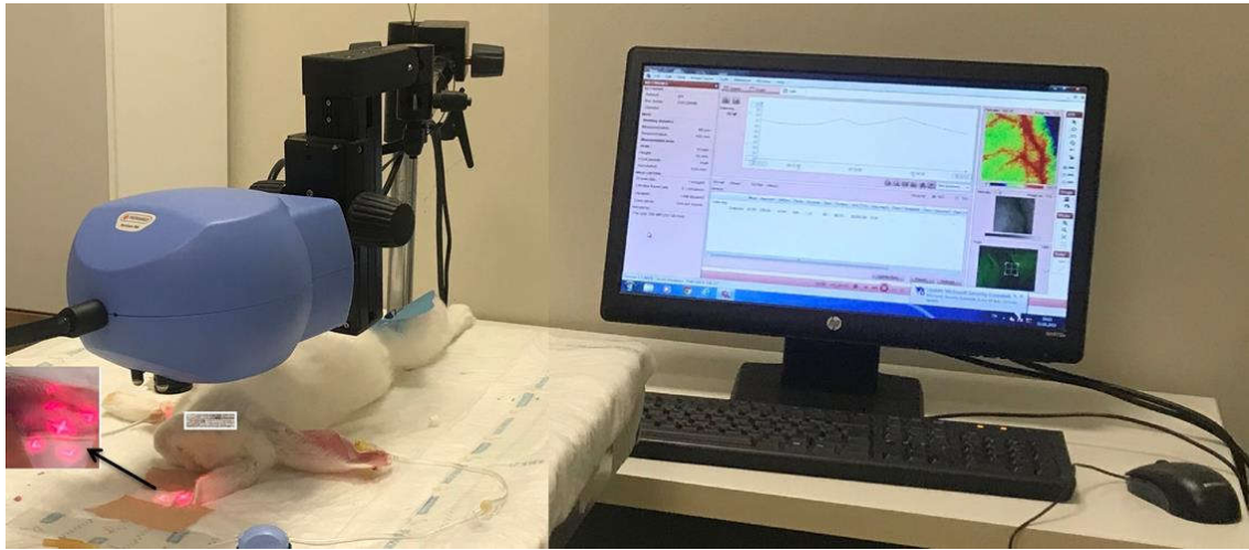
Figure 2.7.3: Laser Speckle Imaging system was placed onto ear of the rabbit
