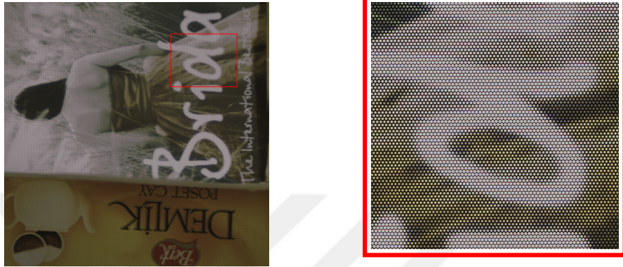
Figure 3.2: Lenslet image of a Lytro camera.
