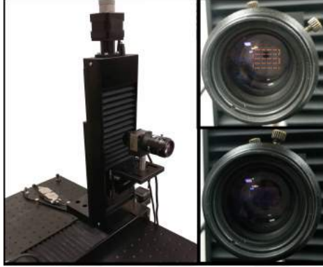
Figure 5.2: Setup for the offline calibration process. (Left) Motorized translation stages and the camera. (Right Top) Narrow aperture opening for perspective images. The camera is moved as illustrated on lens for different perspective images. (Right Bottom) Wide aperture opening for the central image.
