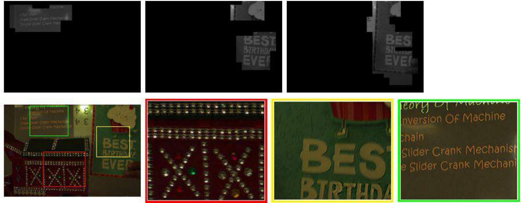
(c) The mean-shift clustering bandwidth is 5.0. (Top) Clustered regions. (Bottom) Final deblurred image and zoomed-in regions.
