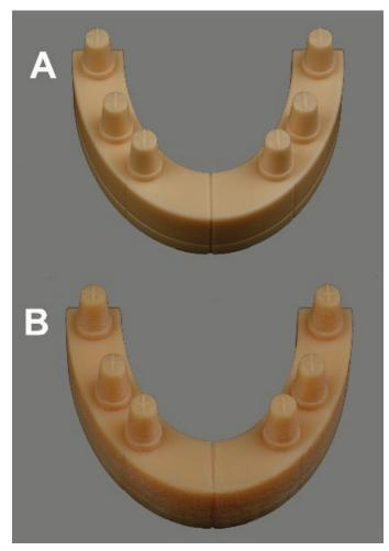
*Figure 1.* The 3D printed models using DLP technology (A) and PolyJet technology (B).
