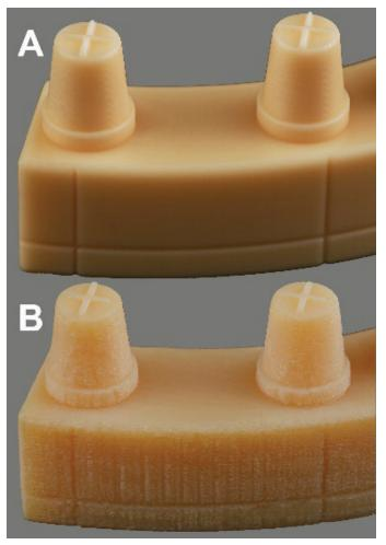
**Figure 4.** The surface quality of 3D printed models. DLP printer used *E-Model material, and PolyJet printer used VeroDentPlus material during* the production of the models. DLP model has a smooth surface, and in contrast to DLP, PolyJet model has a rough surface. A:DLP, B:PolyJet.
