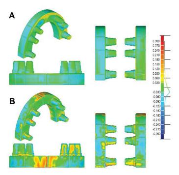
**Figure 2.** The color maps display the discrepancy between the printed models and the master model. The scale bar ranges from -300 to 300  $\mu$ m. Light blue through dark blue color (-30 to -300  $\mu$ m) indicates the printed model is smaller than the master model; green color shows difference  $\pm$ 30  $\mu$ m between printed model and master model; yellow to red color (+30 to +300  $\mu$ m) indicates printed model is larger than the master model. A: DLP, B: PolyJet.
