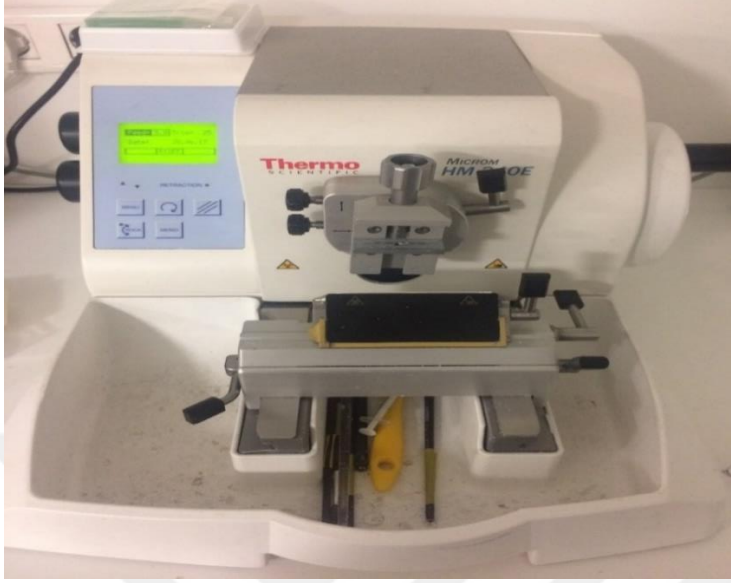
Resim 5.2.1. Mikrotom (Thermo Scientific, HM 340E)
