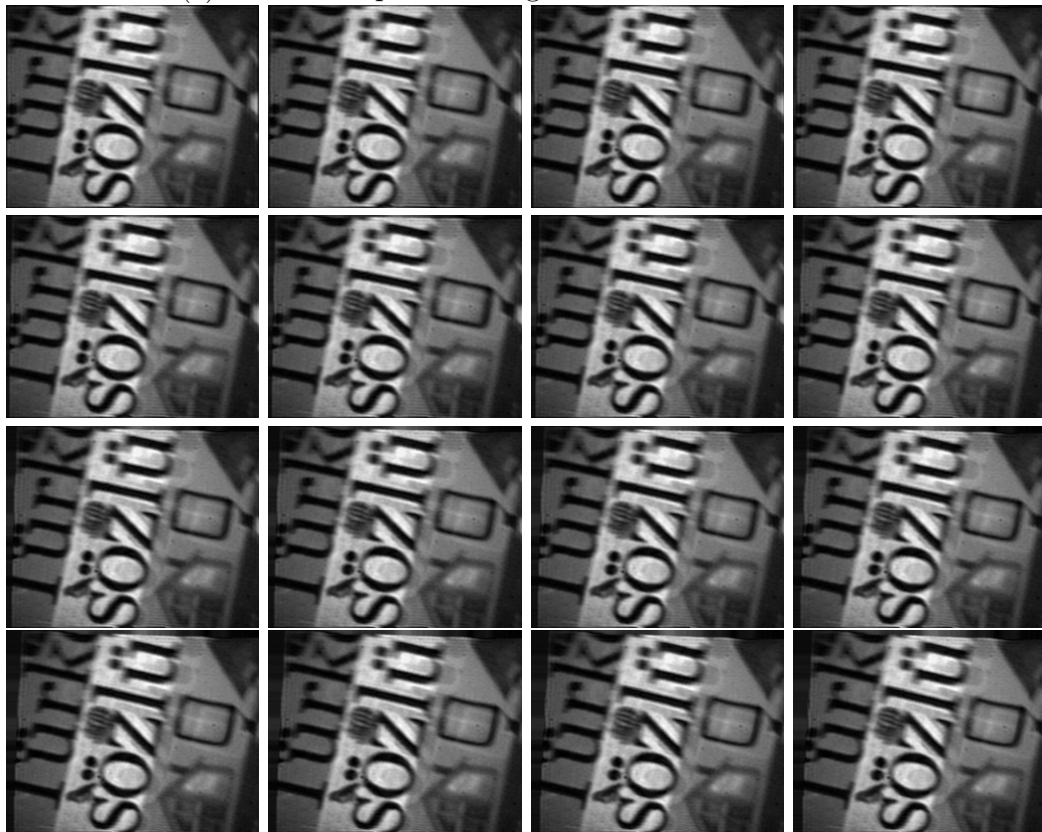
(d) Intermediate frames obtained by interpolating the optical flow vectors.
