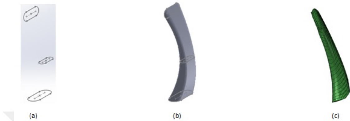
Figure 6.4: a) Sketch of ACL cross-sectional areas b) ACL after loft feature c) ACL in ABAQUS
