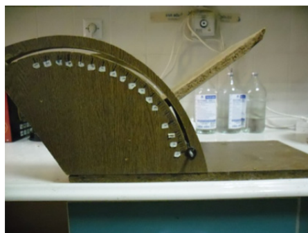
Figure 1 The muscle strength device used to measure the maximum degree at which the rat cannot roll from the device.
