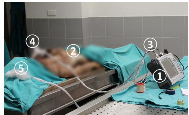
Fig. 3. Experiment setup for the in vivo channel: 1) VNA, 2) human male cadaver, 3) coaxial cables, 4) a novel tapered slot CPW-fed antenna ( in vivo ), and 5) insulated dipole antenna ( ex vivo ).
