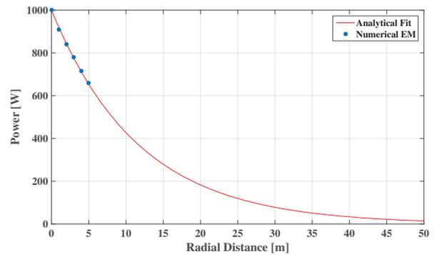
Fig. 6. Net radial power flow versus distance from origin. The dots are from Numerical EM, and the red curve is a fit of the dots to an exponential expression.
