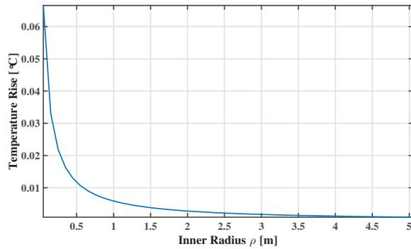
Fig. 4. Temperature rise in a shell of thickness 10 cm and height  $L = 1$  [m].
