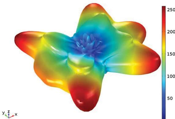
Fig. 10. Far-field pattern due to a radiating Magnetron over a pyramidal reflector array.
