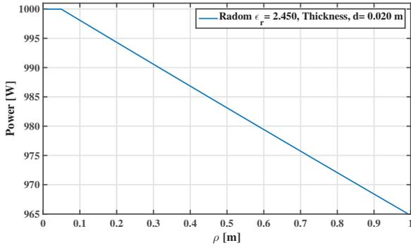
Fig. 3. Power leaving a cylinder of height 1 m and radius  $\rho$ . The thickness of the radome is 2 cm and its dielectric constant is 2.45.
