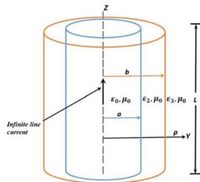
Fig. 1. An infinitely long electric current radiating inside a radome surrounded by infinite calcite medium.
