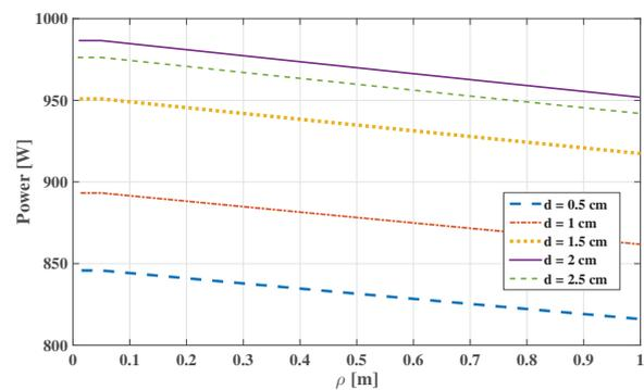
Fig. 2. Power leaving a cylinder of height 1 m and radius  $\rho$ , where  $d$  is the thickness of the radome.
