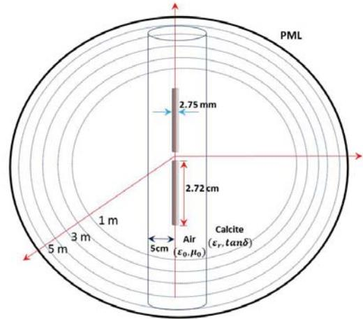
Fig. 5. The model used in COMSOL showing a dipole antenna and the 5 fictitious circles.
