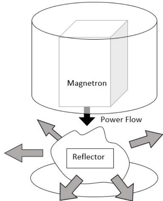
Fig. 8. A section of the microwave heating system where a Magnetron is radiating into an open cavity with a reflector.
