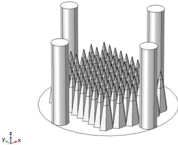
Fig. 9. A pyramidal reflector array designed in COMSOL to reflect power radially outwards.
