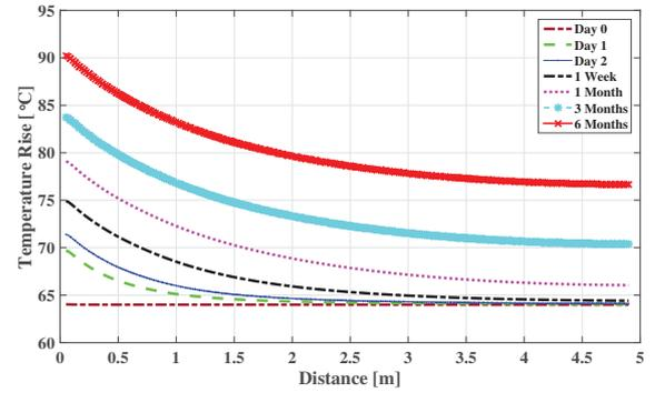
Fig. 7. Temperature variation in calcite (assumed values:  $\epsilon_r = 4$ ,  $\tan\delta = 0.003$ ) with standard thermal conductivity 5.526 [W/(m-k)] and 6 months of constant heating using three 1000 W sources. The initial temperature is taken to be 64°C.
