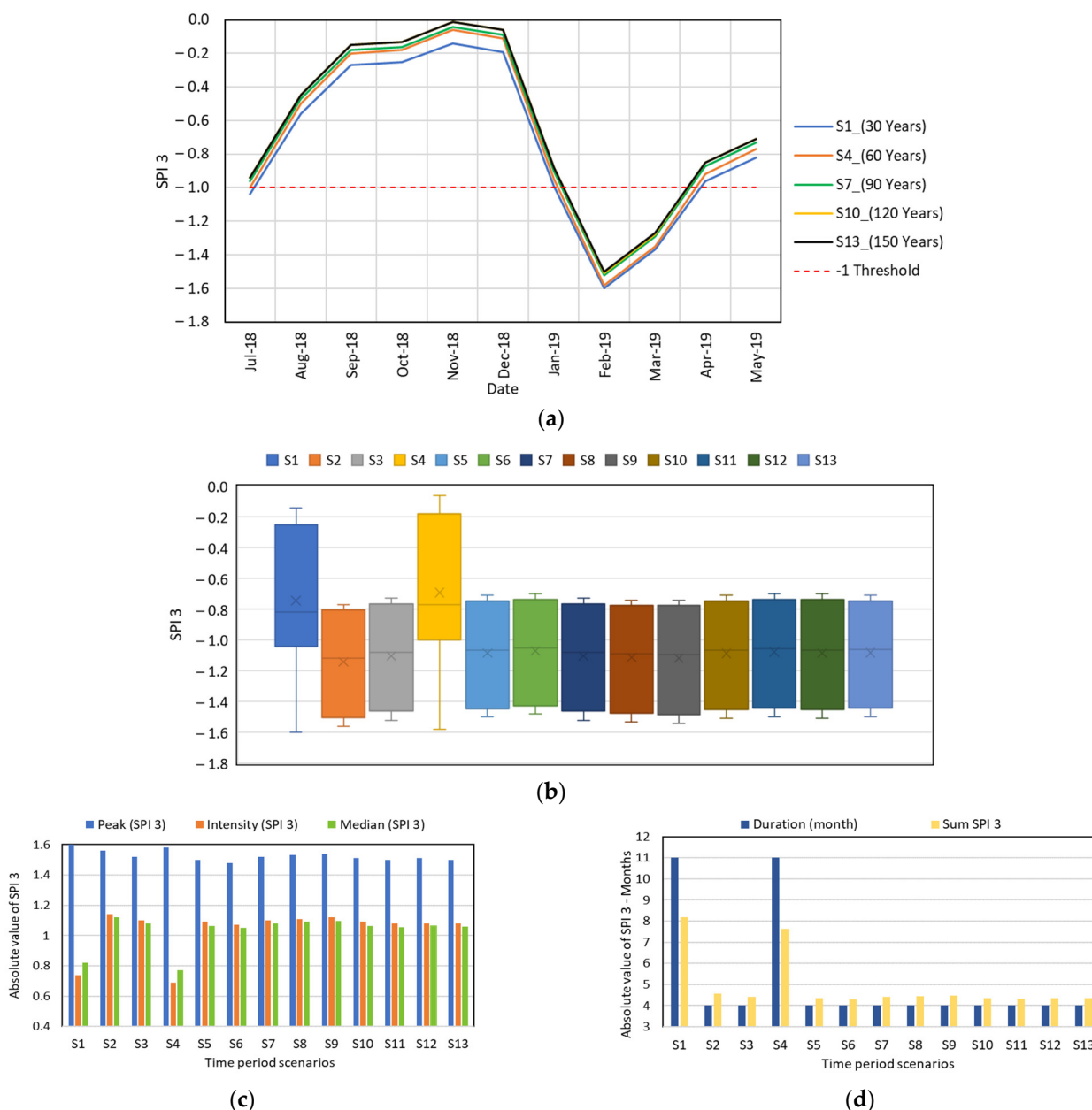
Figure 8. Potential drought characteristics for SPI 3 for the second selected drought event (July 2018–May 2019). (a) The difference between selected scenarios based on SPI 3, (b) the box-and-whisker plot for SPI 3 values, (c) the difference between all time period scenarios using the peak, intensity, and median values, (d) the difference between all time period scenarios using drought duration and the absolute summation of SPI 3 values.
