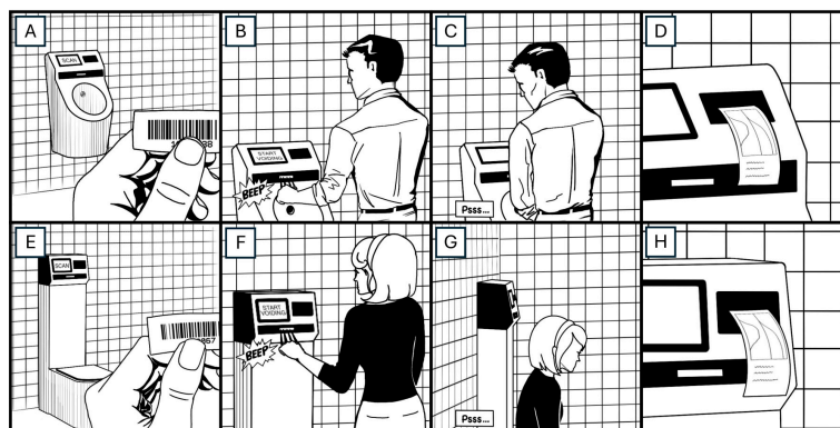
Figure 1. Usage of the portable uroflowmetry. Participants are provided with a unique barcode before entering the restroom (A,E). After scanning the barcode (B,F), the device initiates data recording. Participants can commence voiding within the subsequent minute (C,G). Upon completion of voiding, the device automatically prints the results out, followed by self-cleaning (D,H).
