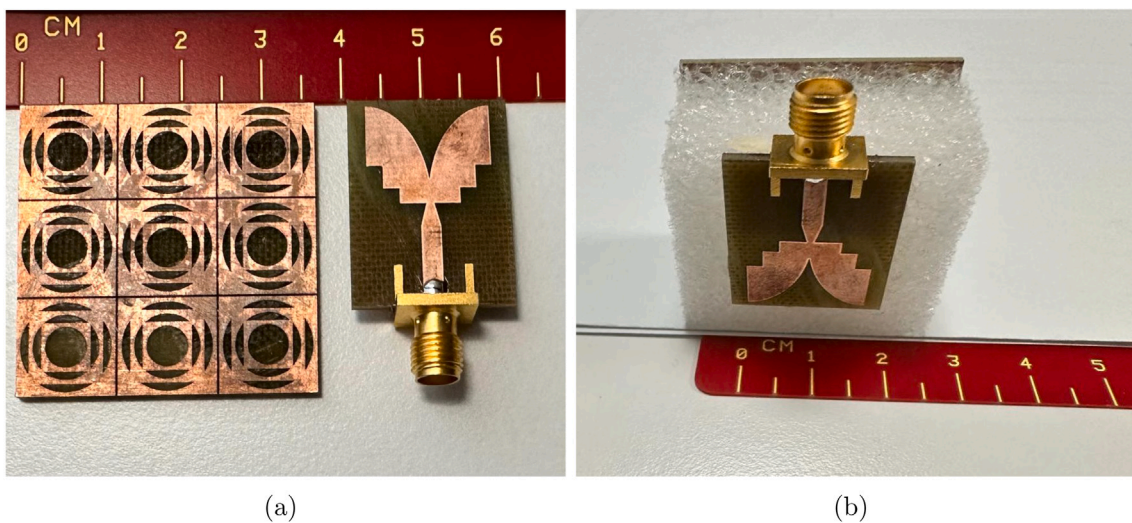
Fig. 12. Fabricated prototype of FSS-integrated UWB antenna (a) before assembly (b) after assembly.
