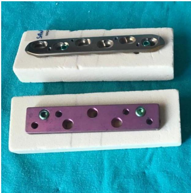
**Fig. 1** Osteoporotic bone model prepared with novel and classical locking plates fixed with 2 screws
