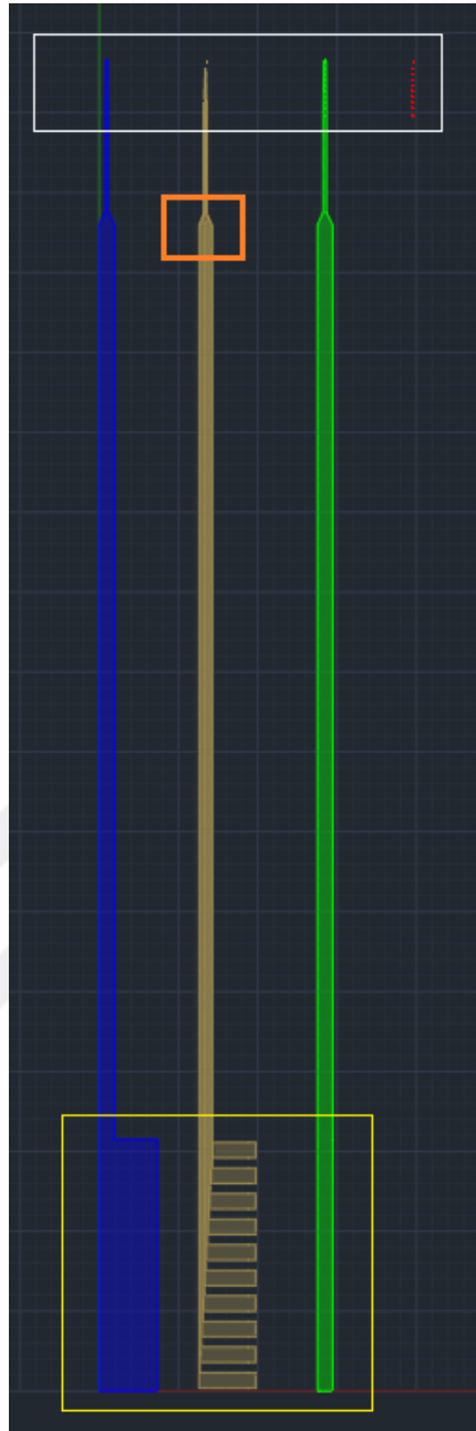
Figure 5.6: Mask design for 4 layers for each microelectrode array. The white box indicates the end of the microelectrode array that penetrates the brain tissue, and the yellow box indicates the part that will be connected to the ZIF connector. A zoomed-in view of the white box is shown in Figure 5.2 , a zoomed-in yellow box is shown in Figure 5.3 , and a zoomed-in orange box is shown in Figure 13. The DXF format drawing file of the image can be downloaded from the link https://1drv.ms/u/s!AsMDMspJ-A9ihvUflZExuGIUm_P1eA?e=eR2G9w .
