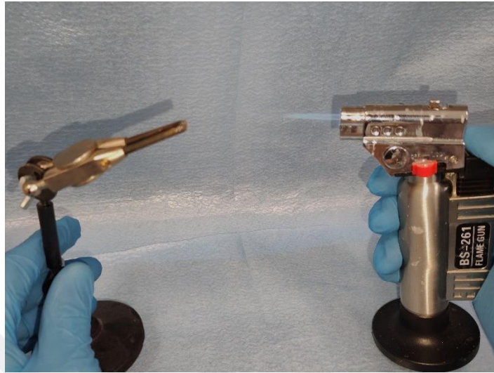
Figure 5.14. Burning adhesive on bracket base with direct torch flame.
