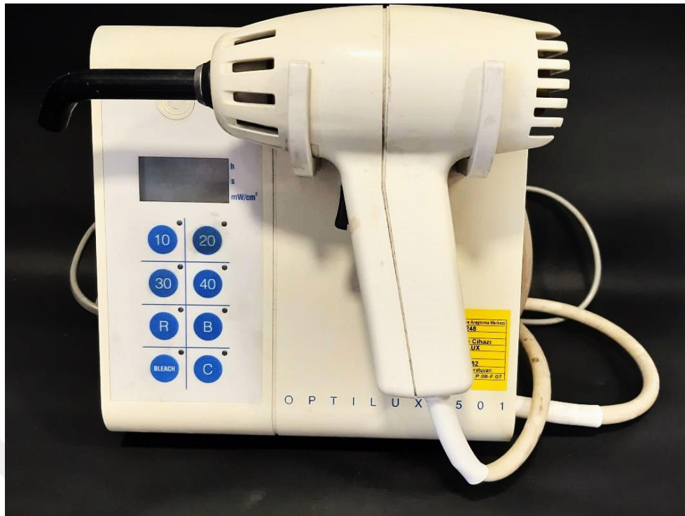
Figure 5.3. Optilux 501 Light Curing Unit.
