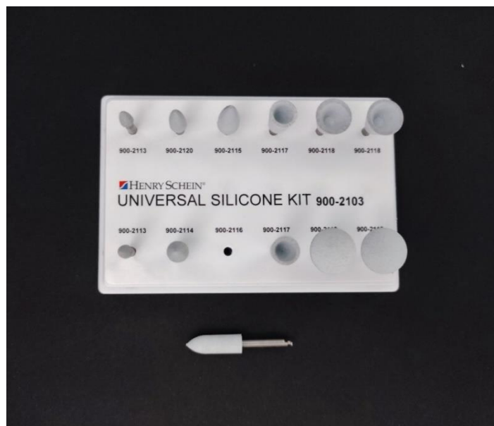
Figure 5.11. Henry Schein Universal Silicone Kit and the bur used (900-2116).
