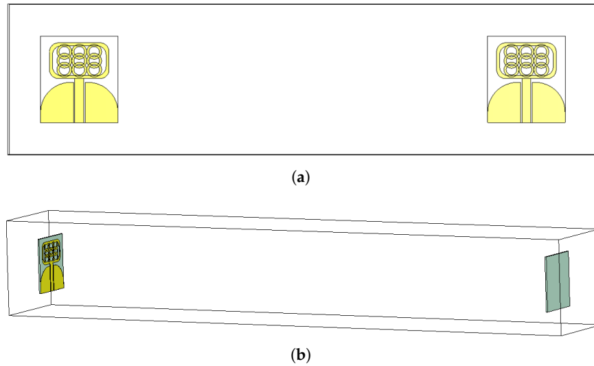
Figure 11. Time-domain analysis configurations: (a) side-by-side and (b) face-to-face.
