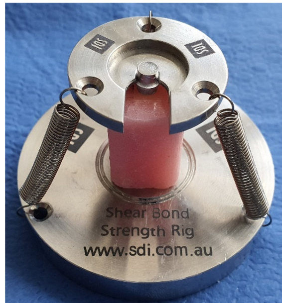
Figure 1. Image of a specimen in the SDI SBS Rig test apparatus.
