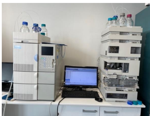
Figure 2. High performance liquid chromatography device (Agilent 1100 HPLC)
