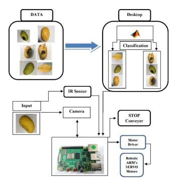
Figure 3. Block diagram indicating training to deployment process.
