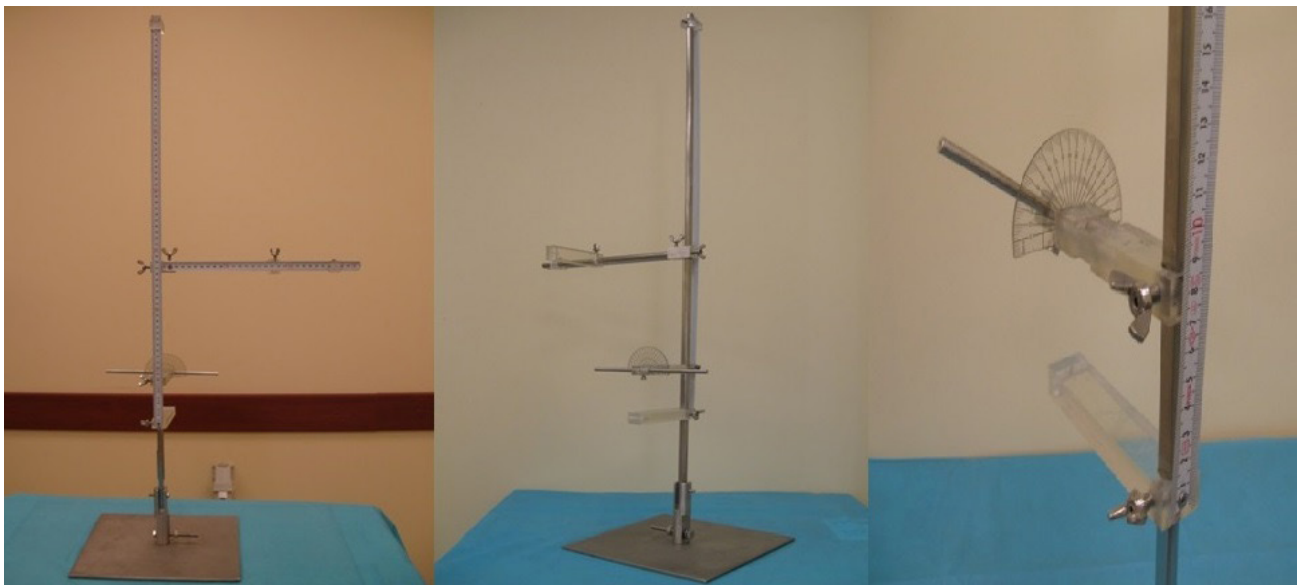
Figure-2. Picture showing the routing device, that is designed according to basic principles of endoscopic transforaminal lumbar disc surgery (AP and antrolateral view: Left and middle respectively). The routing device includes stainless steel bolt at the mid-point of the stainless steel table. U-channel joint is placed in this bolt. The stainless steel rod forms Y axis and passes through the U-channel joints. One side of the Y axis rod is flat in order to have markers stabilized on the rod at 90°. On the other side of the rod, a ruler is placed to make measurements (right).
