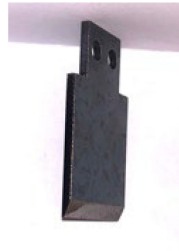
Figure 3. Specially made tip for Universal Testing Machine.
