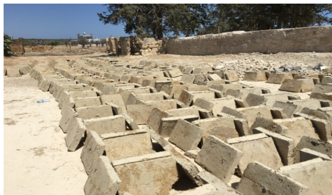
Figure 4. Adobe mud area (mud, pouring into the wooden moulds, removing from the wooden moulds, leaving to drying under the sun)
