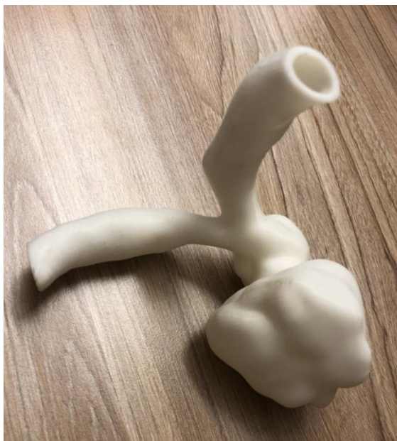
Figure 3.17 A pediatric pulmonary artery lumen prototype printed on an FDM printer. The wall thickness is obtained from the CT dataset with image processing tools due to the pixel color difference.
